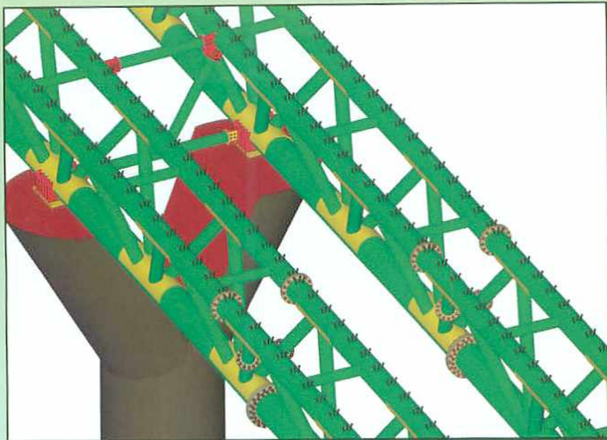
Figure 2: Bottom pipe of each truss rests on arm of "wood-chopped" Y-shaped pier. Tubular diaphragm connects the two trusses at each pier
